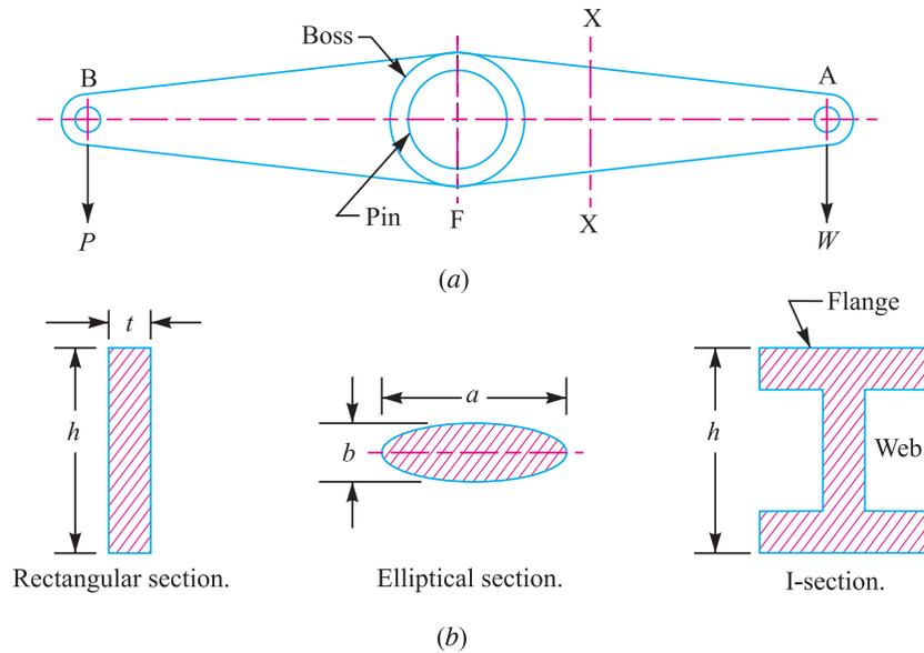
Fig. 15.4. Cross-sections of lever arm (Section at X-X).
