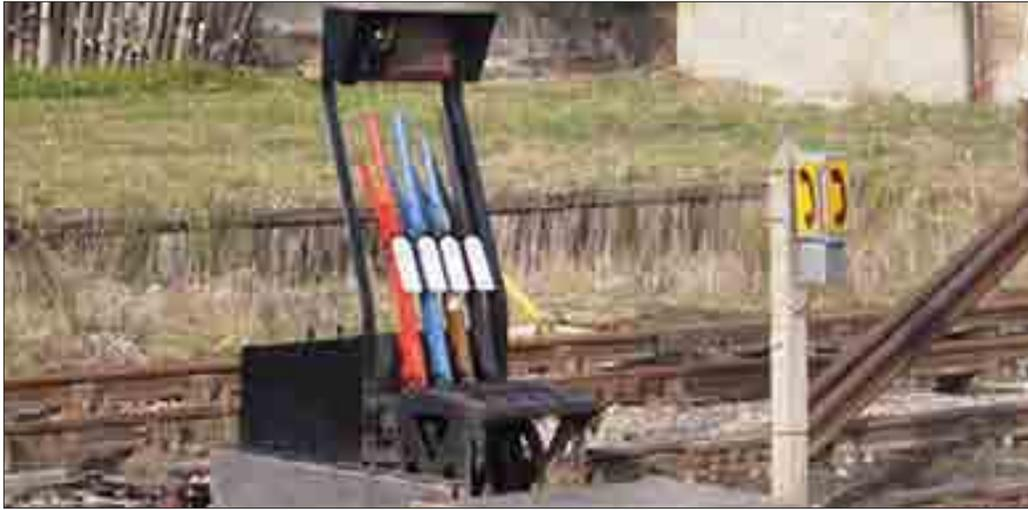
These levers are used to change railway tracks.
